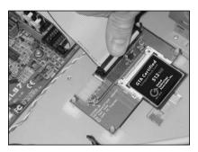
Attaching the IDE Cable to the Compact Flash IDE Adapter Board
